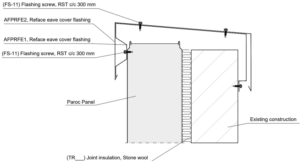
This detail has been done to help architects, engineers and installers when using PAROC panels. Before using this detail, check latest version at [www.parocpanels.com](http://www.parocpanels.com)
