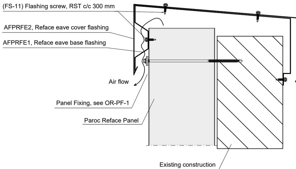
This detail has been done to help architects, engineers and installers when using PAROC panels. Before using this detail, check latest version at [www.parocpanels.com](http://www.parocpanels.com)
