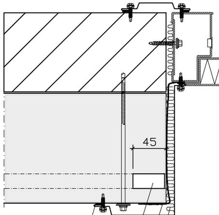
(TT-33) Flashing sealant tape
